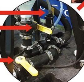
Valve ON is when lever is parrallel to fluid line.
